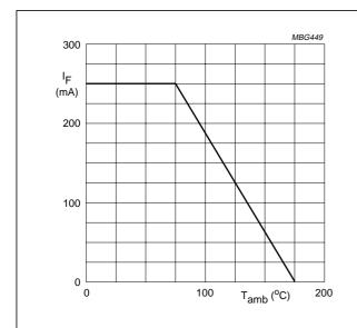
Device mounted on a FR4 printed-circuit board; lead length 10 mm.
