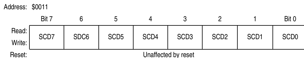
Figure 9-8. SCI Data Register (SCDR)
