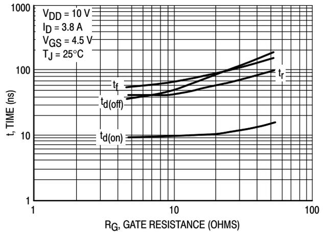
**Figure 11. Resistive Switching Time Variation versus Gate Resistance**
