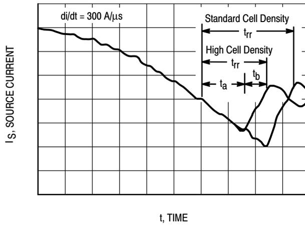
Figure 13. Reverse Recovery Time ( $t_{rr}$ )
