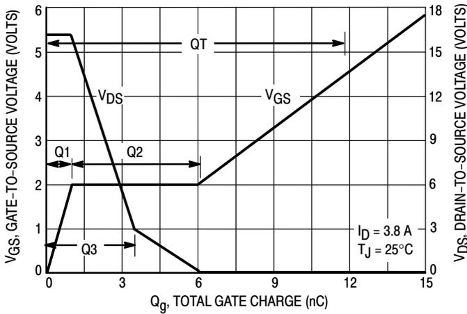
**Figure 10. Gate-To-Source and Drain-To-Source Voltage versus Total Charge**
