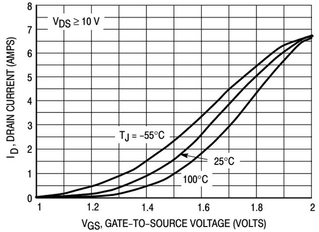
Figure 4. Transfer Characteristics
