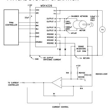
This is a diagram of a typical application of the MSK4226. The design Vcc voltage is +12 volts and should have a good low ESR bypass capacitor such as a tantalum electrolytic. The digital inputs can come from a microprocessor or any type of PWM controller. The controller will use the current sense signal to either control current through PWM, current limit the bridge, or both.
