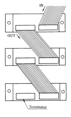
Since the signal contact can be engaged or disengaged, the contact can be used in combination with the cable type and the terminator as illustrated on the left.
