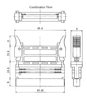
NOTE: This product can be installed in FX2M3-128S8-RC. Applicable cable: 1.27 pitch flat cable AWG28 (7/0.127) insulation covering diameter 0.9mm<UL2651>
