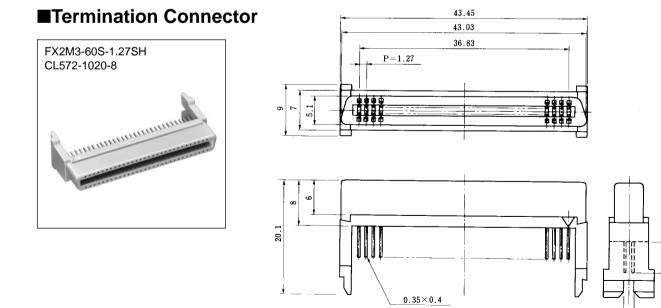
NOTE: The locking type is prepared for the termination connector. Contact the HRS PCC Technical Department for details. 5.5
