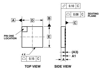
DIMENSIONS AND TOLERANCING PER ASME Y14.5M, 1994. DIMENSIONS IN MILLIMETERS. COPLANARITY APPLIES TO THE LEAD, DIMENSION B, AND EXPOSED PAD. 3. MILLIMETERS
