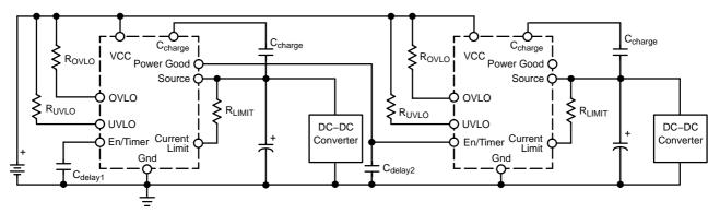
Figure 13. Turn-on Sequencing Using Power Good Signal
