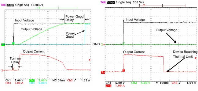
Figure 9. Turn-on Waveforms for 3300 µF Load Capacitors
