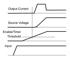
Figure 2. Timing Diagram for External Enabled Delay
