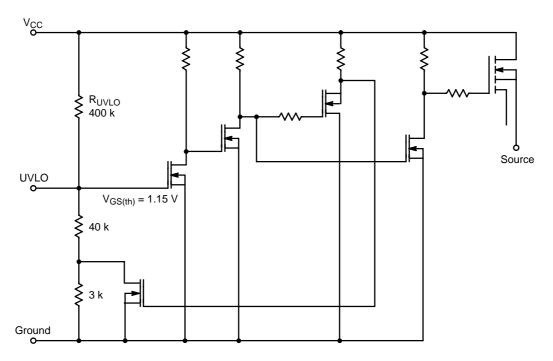
Figure 17. Equivalent Undervoltage Lockout Circuit
