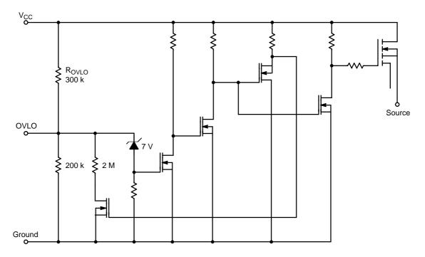
Figure 18. Equivalent Overvoltage Lockout Circuit
