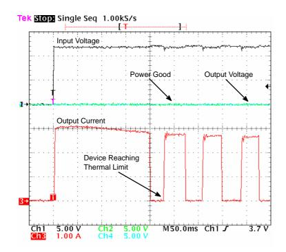
Figure 11. Turn–On Waveforms for Shorted Output, Auto–Retry Device
