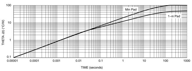
Figure 19. Thermal Transient Response
