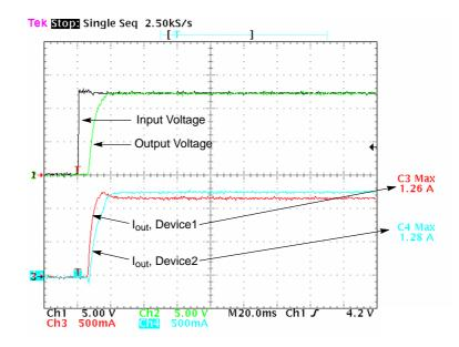
Figure 15. Turn-on Waveforms for Parallel Operation
