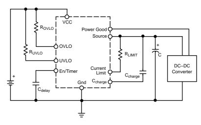
Figure 8. Typical Applications Circuit
