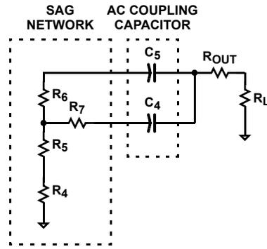
FIGURE 4. SAG NETWORK AND AC COUPLING CAPACITORS
