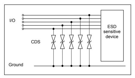
Protection of I/O Lines with discrete CeraDiodes
