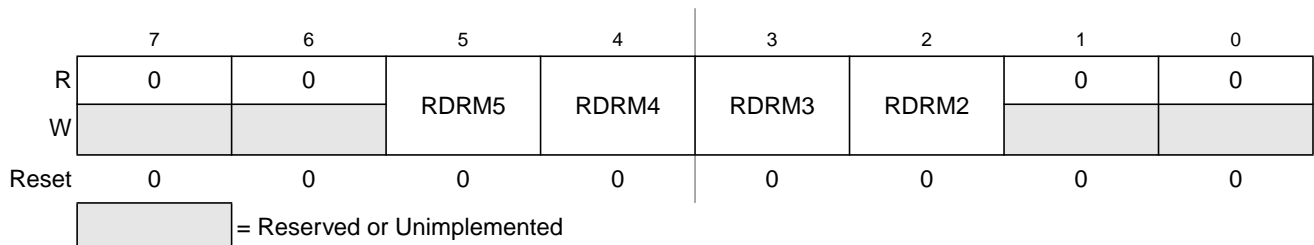
Figure 4-19. Port M Reduced Drive Register (RDRM)
