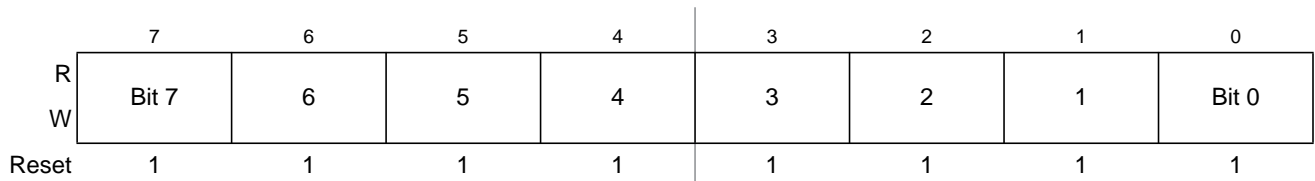
Figure 15-29. PWM Channel Duty Registers (PWMDTY2)
