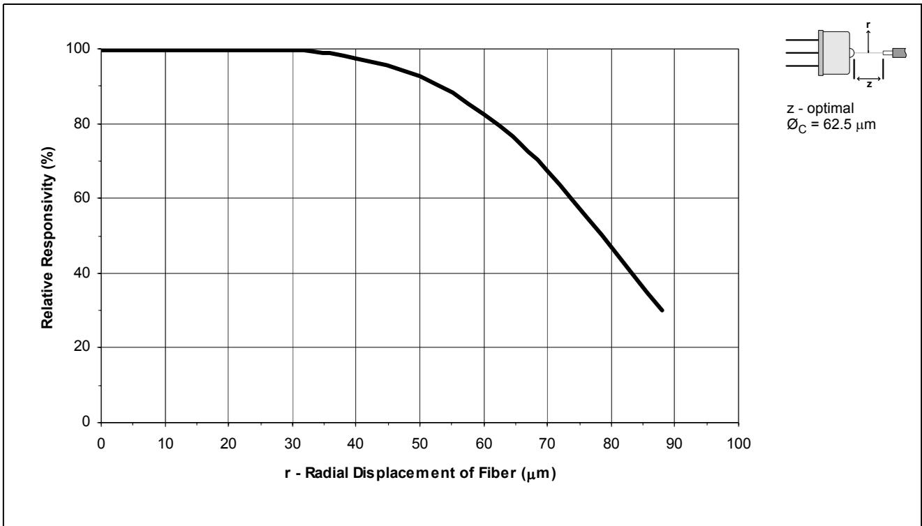
Figure 4 - Relative Responsivity vs. r - Radial Displacement of Fiber
