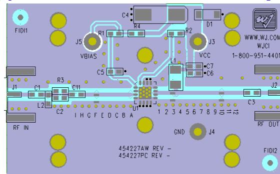
Circuit Board Material: .014" Getek, single layer, 1 oz copper, Microstrip line details: width = .026", spacing = .026"
