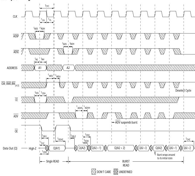
Note: 17. On this diagram, when  $\overline{\text{CE}}$  is LOW:  $\overline{\text{CE}}_1$  is LOW,  $\text{CE}_2$  is HIGH and  $\overline{\text{CE}}_3$  is LOW. When  $\overline{\text{CE}}$  is HIGH:  $\overline{\text{CE}}_1$  is HIGH or  $\text{CE}_2$  is LOW or  $\overline{\text{CE}}_3$  is HIGH.
