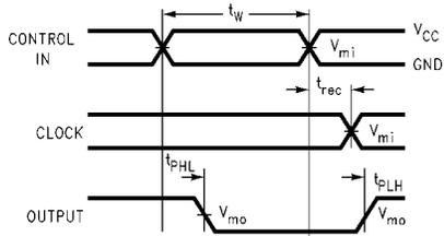
FIGURE 5. Propagation Delay, Pulse Width and  $t_{rec}$  Waveforms
