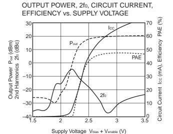
Condition: Vcc1 = Vcc2 = Vbias + Venable = Vcont = 3.0 V, Pin = -20 dBm, with external input and output matching circuit
