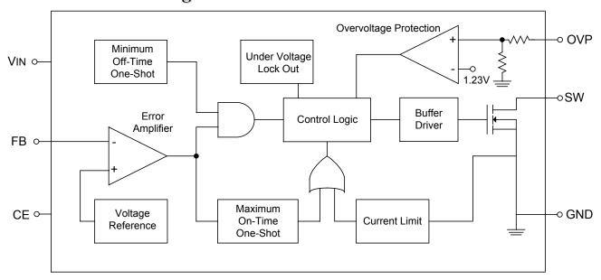
Fig 2. FS8807 Simplified Functional Block Diagram
