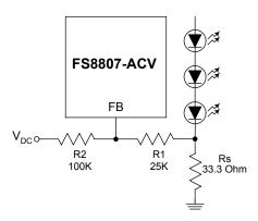
For VDC range from 0V to 2V, the selection of resistors in this figure gives dimming control of LED current from 0mA to 15mA. Following steps are used to select the resistor values:
