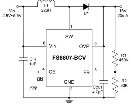
Fig 4. Typical 18V application for line drivers or LCD bias
