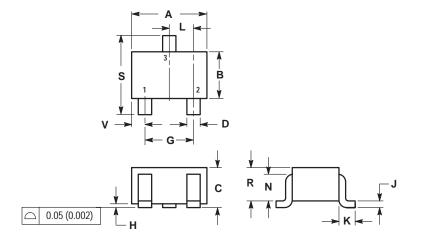
NOTES: 1. DIMENSIONING AND TOLERANCING PER ANSI Y14.5M, 1982. 2. CONTROLLING DIMENSION: INCH.
