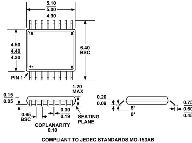
Figure 29. 16-Lead Thin Shrink Small Outline Package [TSSOP] (RU-16)
