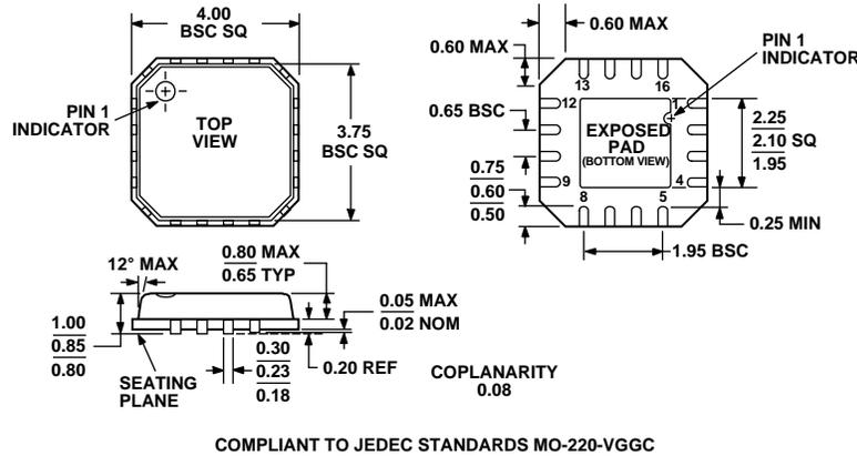
Figure 30. 16-Lead Lead Frame Chip Scale Package [VQ\_LFCSP] 4 mm × 4 mm Body, Very Thin Quad (CP-16-4)
