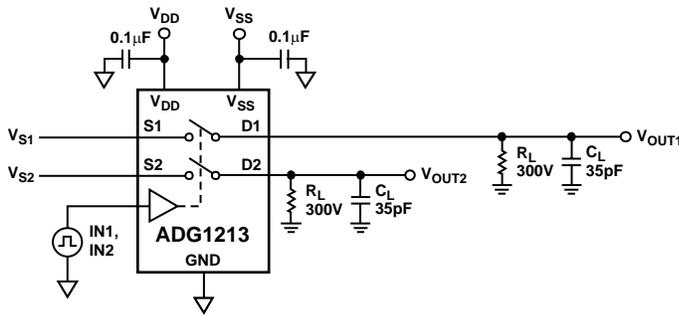
Figure 24. Test Circuit 5—Break Before Make Time Delay
