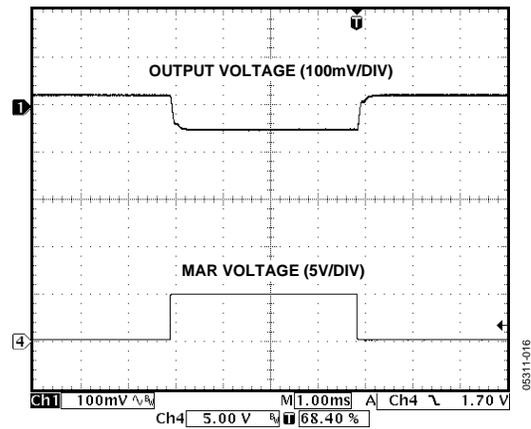
Figure 16. Output Voltage Margin-Down Response
