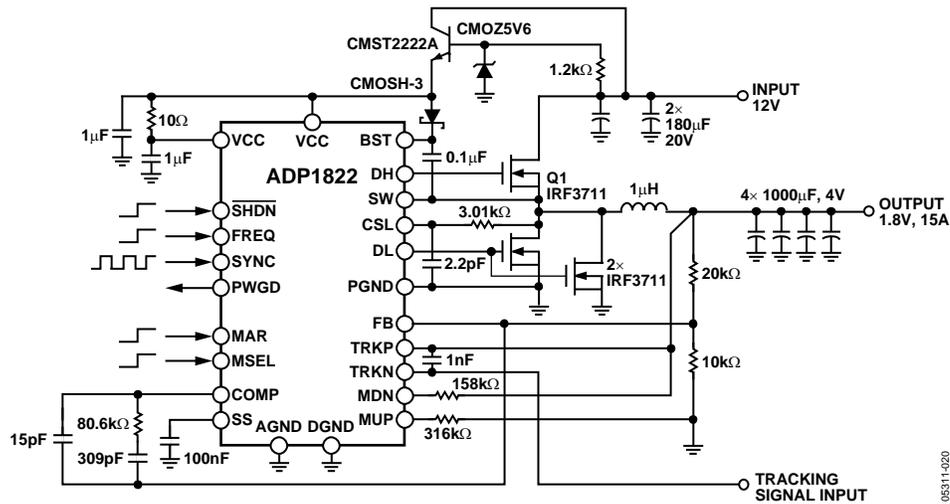
Figure 22. Typical Application Circuit, 12 V Input
