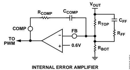
Figure 20. Compensation Using Feed-Forward
