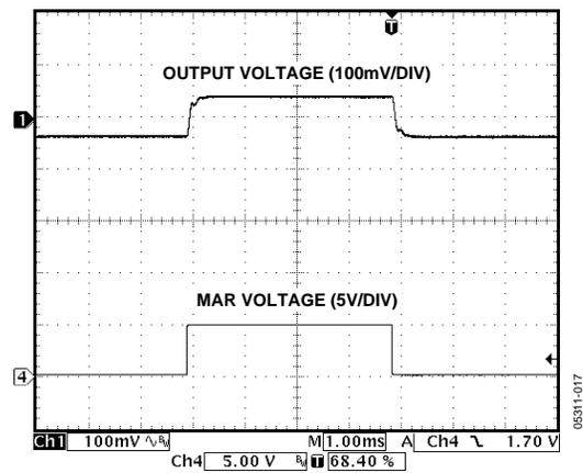
Figure 17. Output Voltage Margin-Up Response
