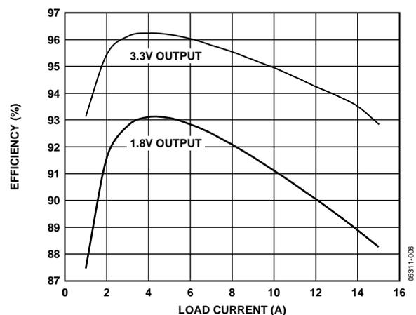
Figure 2. Efficiency vs. Load Current, 5 V Input
