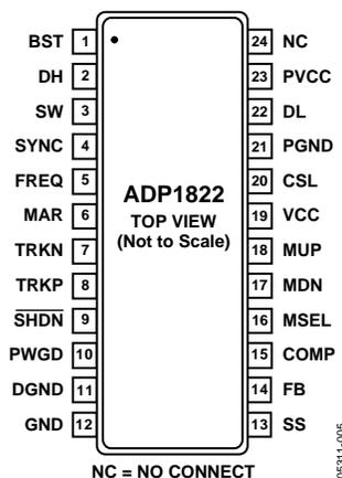
Figure 4. Pin Configuration
