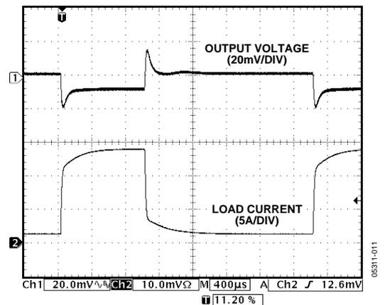
Figure 10. Load Transient Response, 1.5A to 15A
