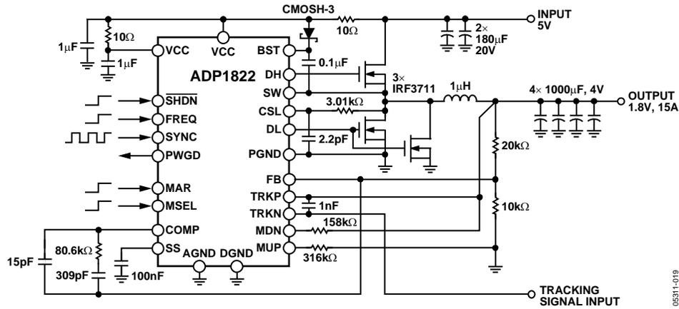
Figure 21. Typical Application Circuit, 5 V Input
