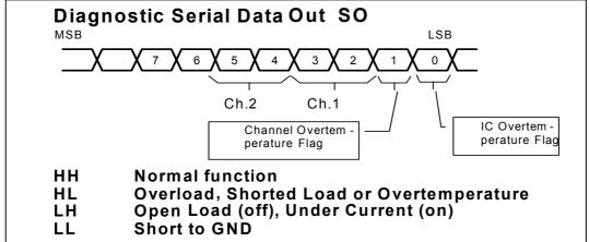
For Full Diagnosis there are two diagnostic bits per channel configured as shown in Figure 1. Bit 6 and bit 7 of the diagnostic register are not used and always H.
