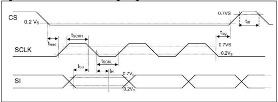
Figure 8: Input Timing Diagram
