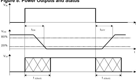
Figure 6: Open load (off) and Short to GND Diagnostics
