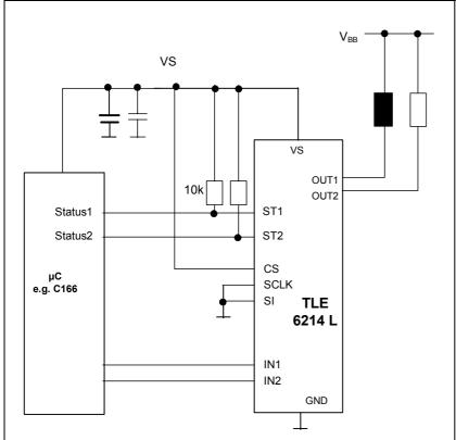
Application Circuit using SPI and Current Sense Output
