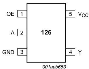
Fig.1 Pin configuration SC-88A; SC-74A.
