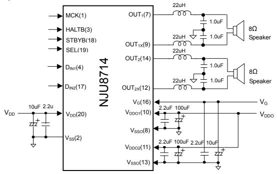
Note 3) De-coupling capacitors must be connected between each power supply pin and GND pin.
