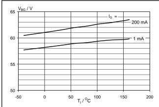
Fig.22. Typical battery to ground clamping voltage.  $V_{BG} = f(T_i)$ ; parameter  $I_G$
