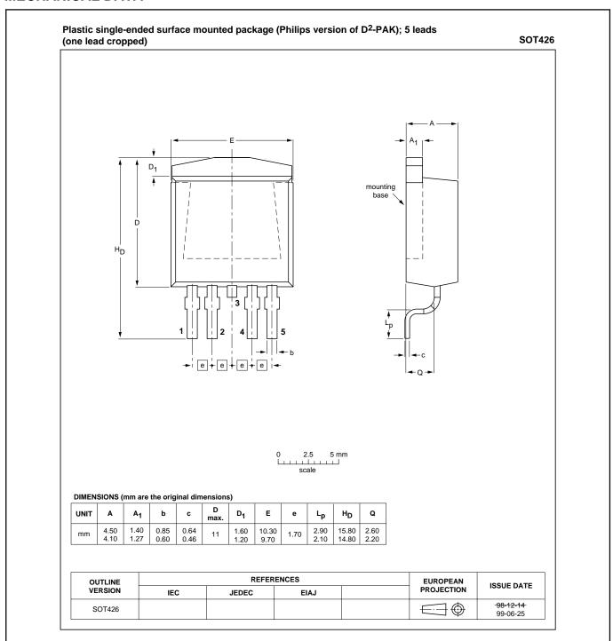
Fig.34. SOT426 surface mounting package<sup>1</sup>, centre pin connected to mounting base.
