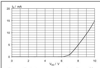
Fig.21. Typical status characteristic,  $T_j = 25$  °C.  $I_S = f(V_{SG})$ ; conditions  $V_{IG} = V_{BG} = 0V$
