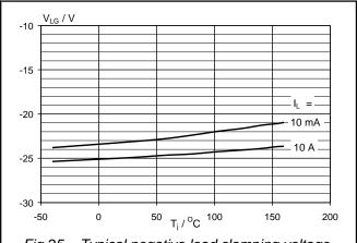
Fig.25. Typical negative load clamping voltage.  $V_{LG} = f(T_j)$ ; parameter  $I_L$ ; condition  $V_{IG} = 0$ V
