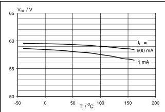
Fig.23. Typical battery to load clamping voltage.  $V_{BL} = f(T_j)$ ; parameter  $I_L$ ; condition  $I_G = 10 \text{mA}$
