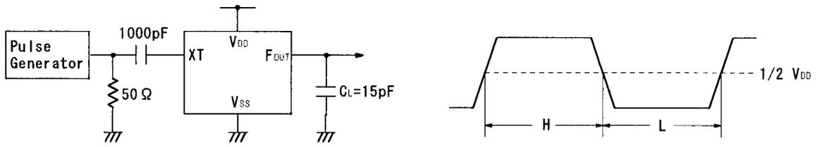
(2) Output Signal Rise/Fall Time ( $C_L=15\text{pF}$ )
