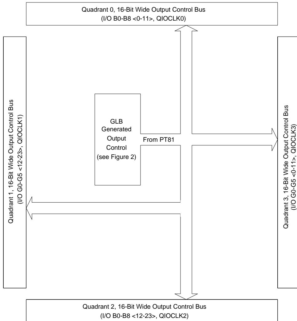
Figure 5. Output Control Bus and Quadrant Organization
