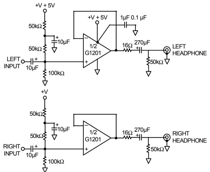
**Figure 2. A Single-Supply, Stereo Headphone Driver**
