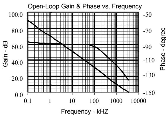
**Test Condition:  $T_A=25^{\circ}\text{C}$ ,  $V+ = 2.5\text{V}$ ,  $V- = -2.5\text{V}$**
