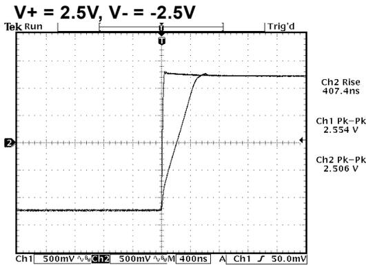
**SR (rising) =  $2.5\text{V}/408\text{ns} = 6.14\text{V}/\mu\text{s}$**
