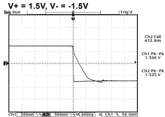
**SR (falling) =  $1.5\text{V}/434\text{ns} = 3.45\text{V}/\mu\text{s}$**
