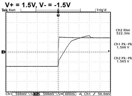
**SR (rising) =  $1.5\text{V}/522\text{ns} = 2.87\text{V}/\mu\text{s}$**
