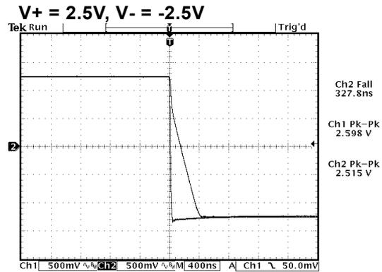
**SR (falling) =  $2.5\text{V}/327\text{ns} = 7.65\text{V}/\mu\text{s}$**
