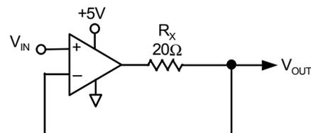
**Figure 1. Output Short-Circuit Protection**
