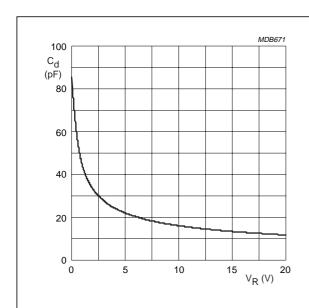
Fig.10 Diode capacitance as a function of reverse voltage; typical values.
