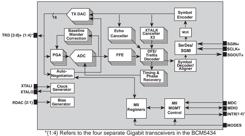
The **BCM5434** consists of four complete 10/100/1000BASE-T Gigabit Ethernet transceivers integrated on a single monolithic CMOS chip. The **BCM5434** is optimized for low power and small footprint size to enable high port density applications. By doubling transceiver port density, lowering system cost, and reducing power dissipation by nearly 50%, the **BCM5434** enables a new class of cost-effective Gigabit Ethernet equipment, driving the delivery of Gigabit bandwidth to the desktop.
