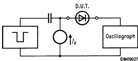
Pulse generator:  $t_p = 5 \mu\text{s}$ ,  $D = 0.05$
