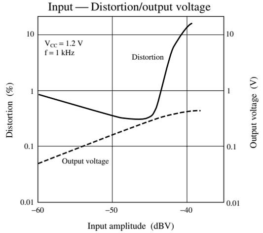
3. Distortion and amplitude characteristics of headphone amp.
