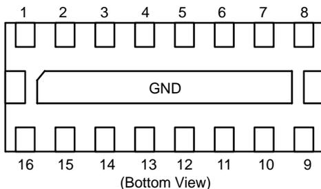
Figure 1. Pin Connections
