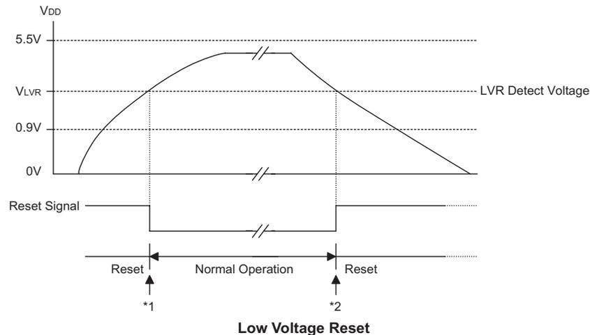
Note: \*1: To make sure that the system oscillator has stabilized, the SST provides an extra delay of 1024 system clock pulses before entering the normal operation.
