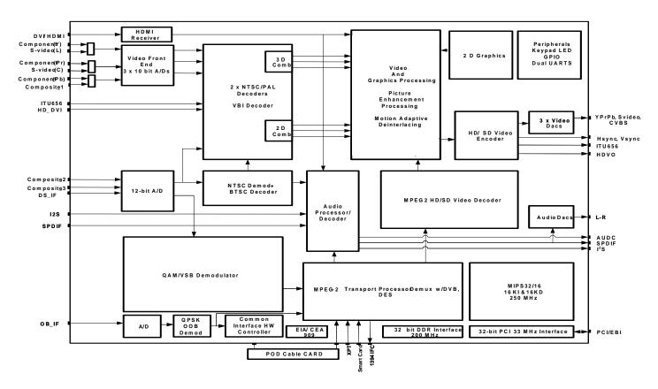
The BCM3560 combines a cable/terrestrial 4/1024-QAM and 8/16-VSB receiver, an out-of-band QPSK receiver, NTSC demodulator, DVI/HDMI receiver, a transport processor, a digital audio processor, a high-definition (HD) MPEG video decoder, 2D graphics processing, digital processing of analog video and audio, analog video digitizer and DAC functions, stereo high-fidelity audio DACs, a 250-MHz MIPS processor, and a peripheral control unit providing a variety of television control functions.
