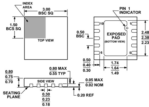
Figure 43. . 10-Lead Lead Frame Chip Scale Package
