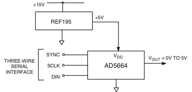
Figure 40. REF195 as Power Supply to the AD5624R/AD5644R/AD5664
