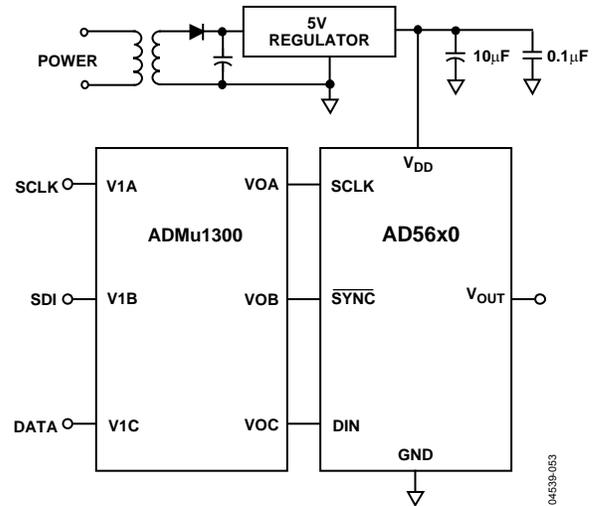
Figure 42. AD5663R with a Galvanically Isolated Interface
