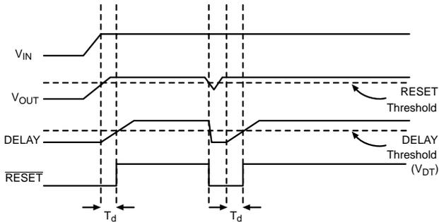
Figure 11. Reset and Delay Circuit Wave Forms
