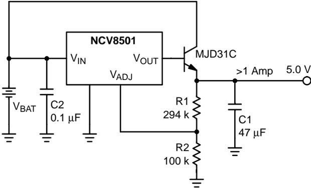
Figure 15. Additional Output Current
