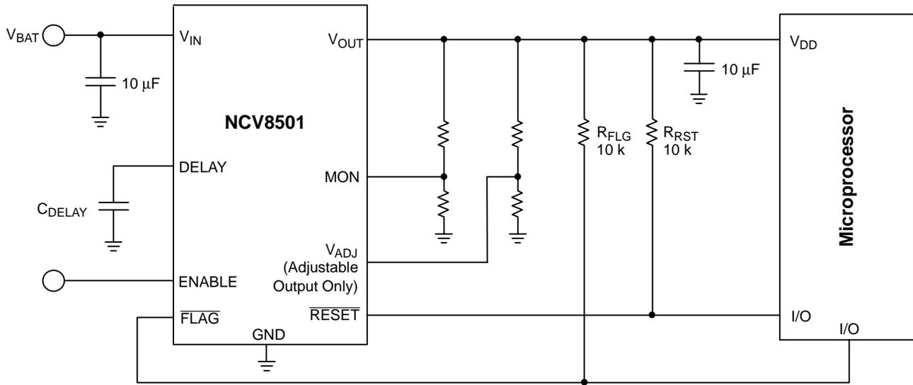
Figure 1. Application Diagram
