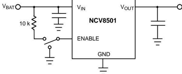
Figure 12. ENABLE Function
