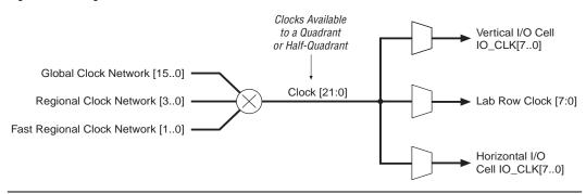
IOE clocks have horizontal and vertical block regions that are clocked by eight I/O clock signals chosen from the 22 quadrant or half-quadrant clock resources. Figures 2–47 and 2–48 show the quadrant and half-quadrant relationship to the I/O clock regions, respectively. The vertical regions (column pins) have less clock delay than the horizontal regions (row pins).
