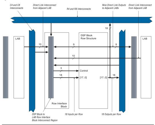
Figure 2-41. DSP Block Interface to Interconnect
