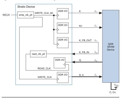
Figure 2-73. QDR SRAM Interfacing
