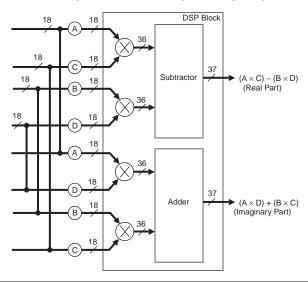
Figure 2–38. Two-Multipliers Adder Mode Implementing Complex Multiply
