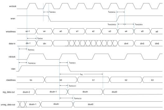
Figure 4–3. Dual-Port RAM Timing Microparameter Waveform
