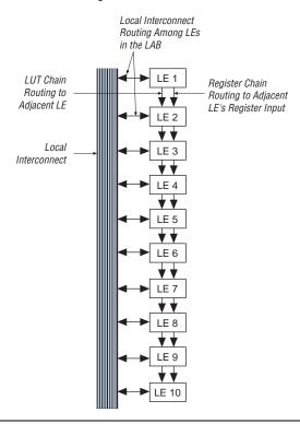
Figure 2-10. LUT Chain & Register Chain Interconnects
