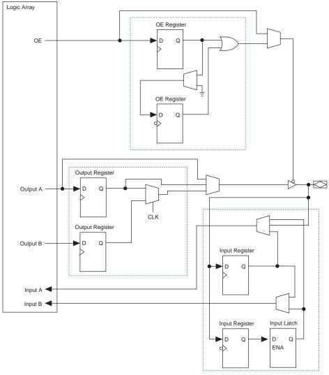
The IOEs are located in I/O blocks around the periphery of the Stratix device. There are up to four IOEs per row I/O block and six IOEs per column I/O block. The row I/O blocks drive row, column, or direct link interconnects. The column I/O blocks drive column interconnects. Figure 2–60 shows how a row I/O block connects to the logic array. Figure 2–61 shows how a column I/O block connects to the logic array.
