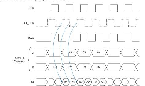
Figure 2-70. Output TIming Diagram in DDR Mode
