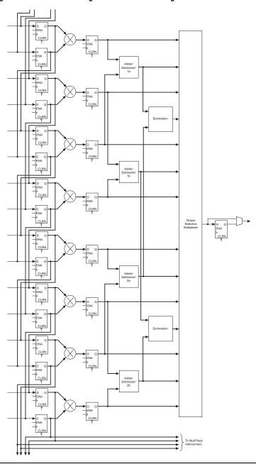
Figure 2–31. DSP Block Diagram for  $9 \times 9$ -Bit Configuration
