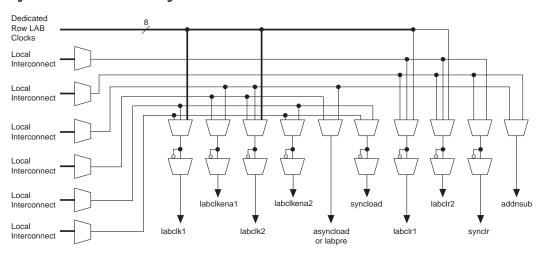
Figure 2-4. LAB-Wide Control Signals
