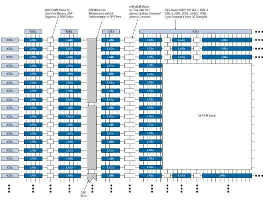
Figure 2–1. Stratix Block Diagram
