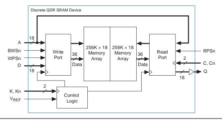
Stratix devices utilize the DDR I/O circuitry for the input and output data bus and the K and Kn output clock signals. Figure 2–73 shows QDR SRAM interfacing from the I/O pin using the DDR I/O circuitry. Stratix devices also support QDR II SRAM at higher clock speeds since the timing requirements for QDR II SRAM are not as strict as QDR SRAM. Altera offers a QDR SRAM Controller Reference Design that can be modified to interface with multiple QDR SRAM devices.
