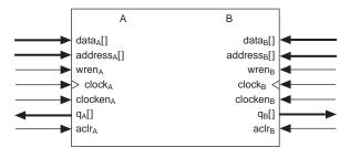
In addition to true dual-port memory, the memory blocks support simple dual-port and single-port RAM. Simple dual-port memory supports a simultaneous read and write and can either read old data before the write occurs or just read the don't care bits. Single-port memory supports non-simultaneous reads and writes, but the q[] port will output the data once
