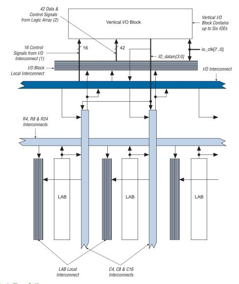
Figure 2-61. Column I/O Block Connection to the Interconnect
