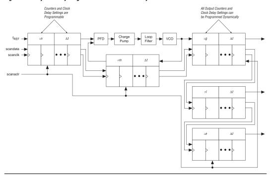
Figure 2-54. Dynamically Programmable Counters & Delays in Stratix Device Enhanced PLLs
