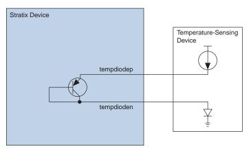
Figure 3-5. External Temperature-Sensing Diode
