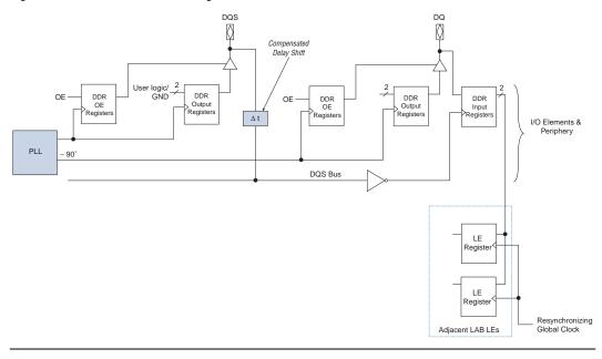
Figure 2-71. DDR SDRAM Interfacing
