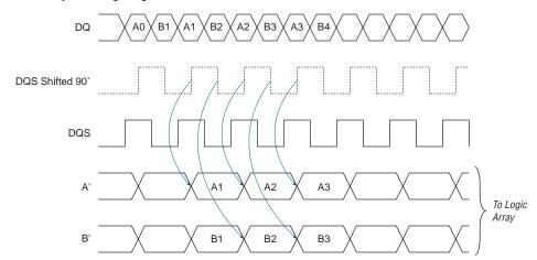
Figure 2-69. Input Timing Diagram in DDR Mode
