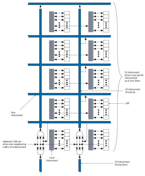
Figure 2–11. C4 Interconnect Connections Note (1)
