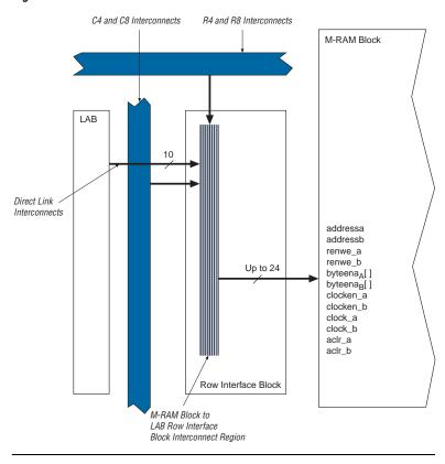
Figure 2-22. M-RAM Row Unit Interface to Interconnect
