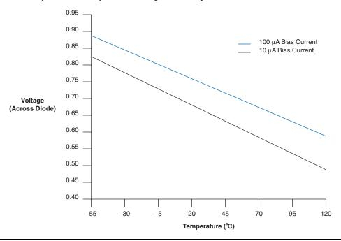
Figure 3-6. Temperature vs. Temperature-Sensing Diode Voltage
