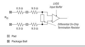
Table 2–35 defines the specification for internal termination resistance for commercial devices.
