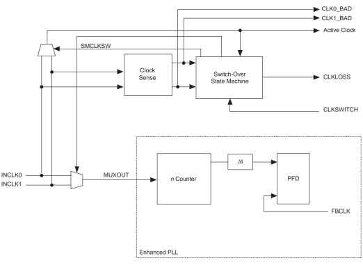
Figure 2-53. Clock Switchover Circuitry
