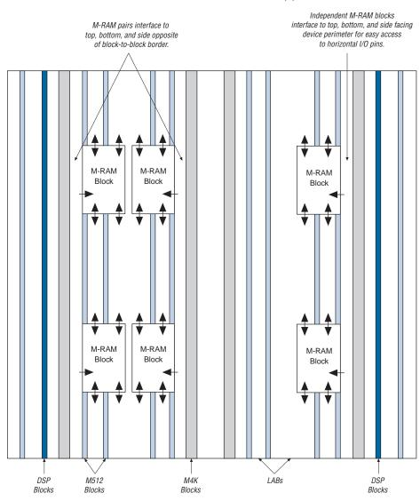
Figure 2–20. EP1S60 Device with M-RAM Interface Locations Note (1)
