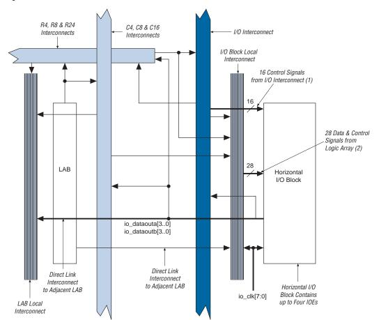
Figure 2-60. Row I/O Block Connection to the Interconnect
