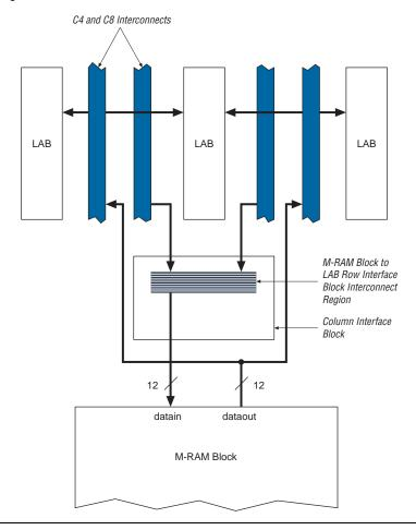
Figure 2-23. M-RAM Column Unit Interface to Interconnect
