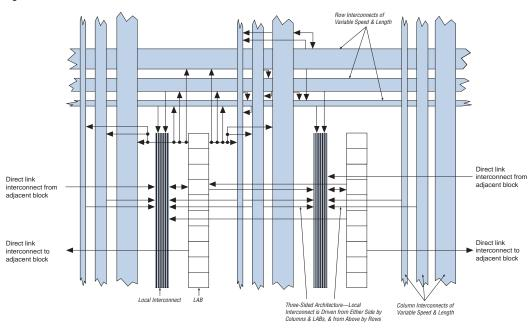
Figure 2-2. Stratix LAB Structure
