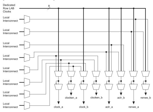
Figure 2-19. M-RAM Block Control Signals
