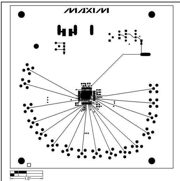
Figure 4. MAX555 EV Kit PC Board Layout—Component Side
