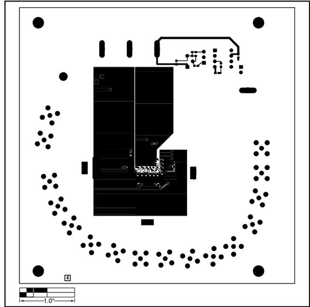
Figure 7. MAX555 EV Kit PC Board Layout—Back Side
