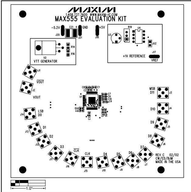
Figure 2. MAX555 EV Kit Component Placement Guide—Component Side
