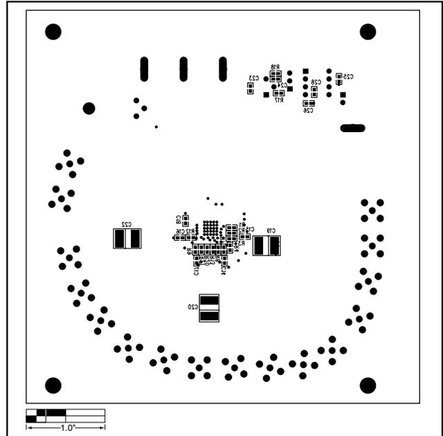
Figure 3. MAX555 EV Kit Component Placement Guide—Back Side
