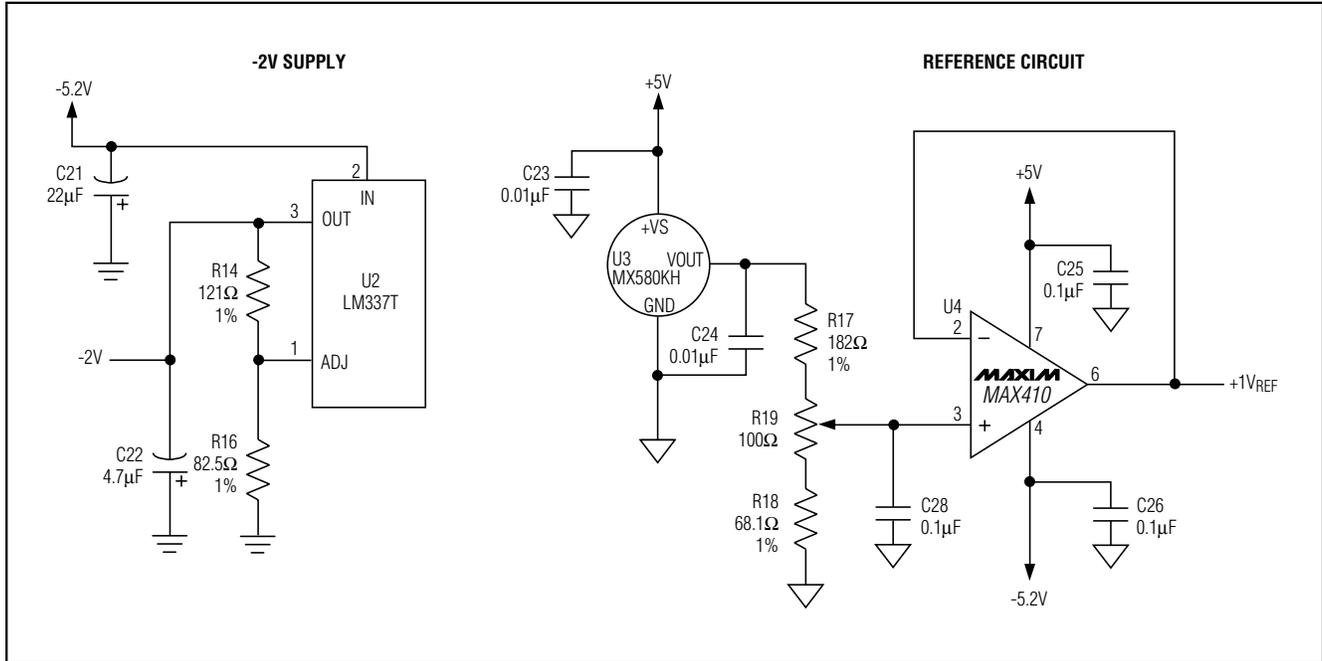
Figure 1. MAX555 EV Kit Schematic Diagram (Sheet 2 of 2)
