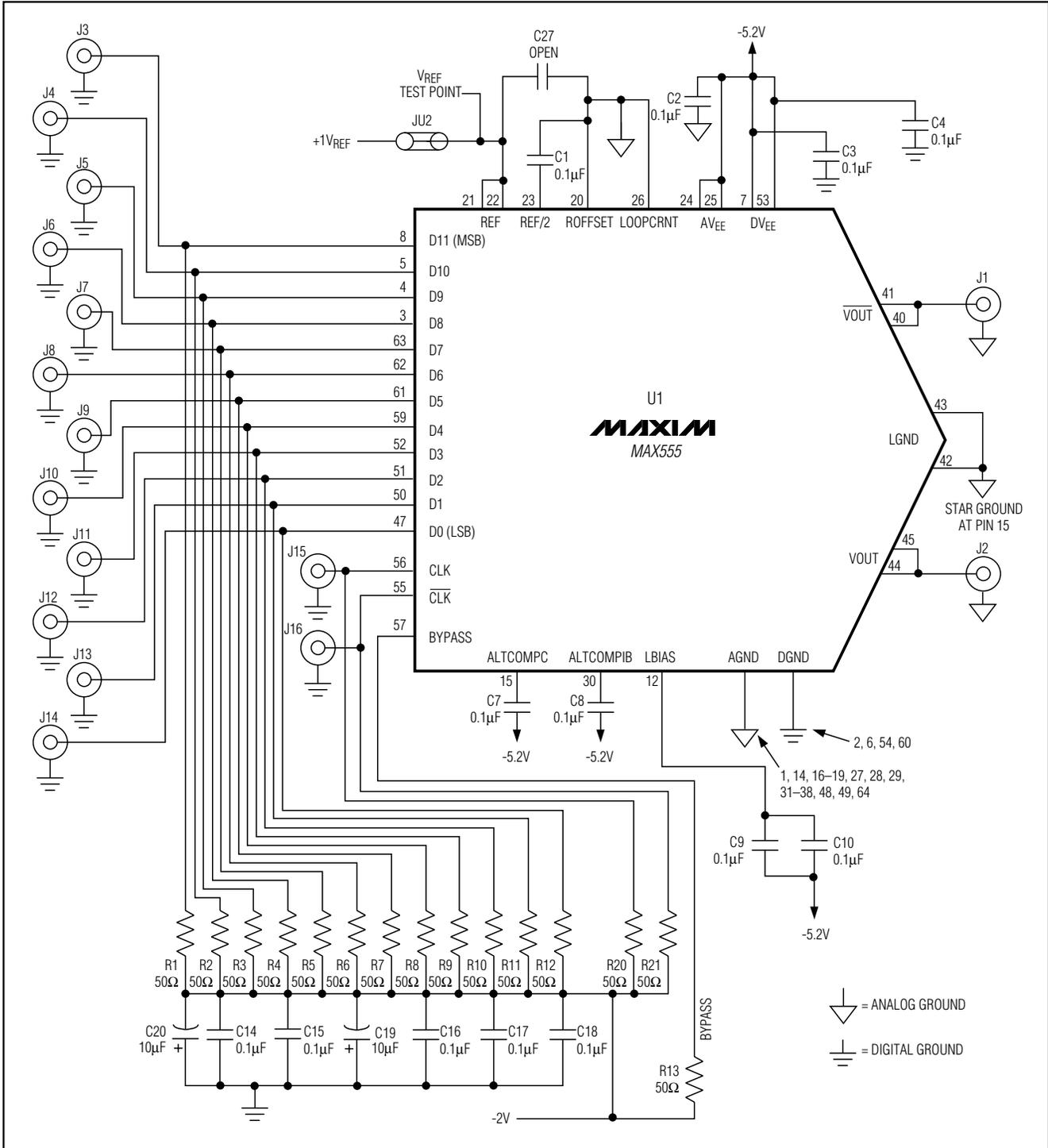
Figure 1. MAX555 EV Kit Schematic Diagram (Sheet 1 of 2)
