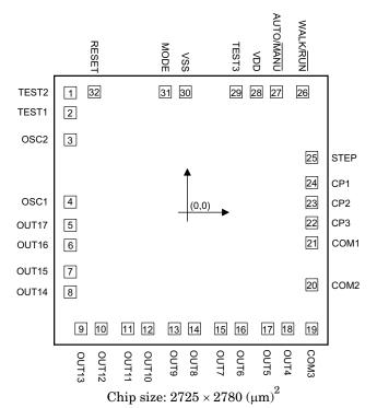
$\ensuremath{^{*}}$  The IC substrate should be connected to VDD in the PCB layout artwork.
