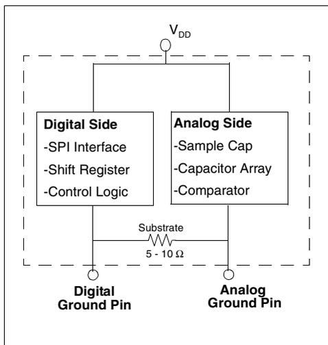
**FIGURE 6-5:** Separation of Analog and Digital Ground Pins.
