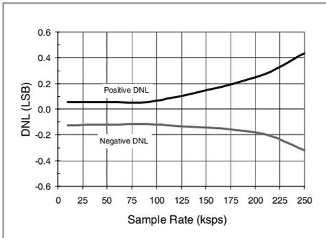
**FIGURE 2-8:** Differential Nonlinearity (DNL) vs. Sample Rate.
