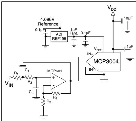
**FIGURE 6-3:** The MCP601 Operational Amplifier is used to implement a 2nd order anti-aliasing filter for the signal being converted by the MCP3004.
