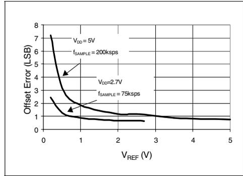
**FIGURE 2-18:** Offset Error vs.  $V_{REF}$ .
