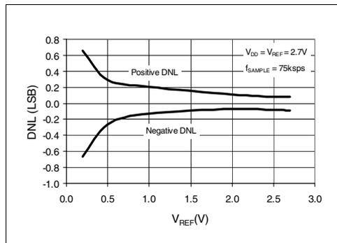
**FIGURE 2-12:** Differential Nonlinearity (DNL) vs.  $V_{REF}$  ( $V_{DD} = 2.7V$ ).
