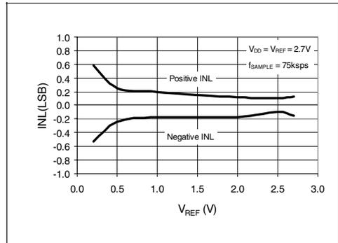
**FIGURE 2-5:** Integral Nonlinearity (INL) vs.  $V_{REF}$  ( $V_{DD} = 2.7V$ ).
