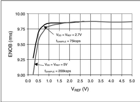
**FIGURE 2-25:** Effective Number of Bits (ENOB) vs.  $V_{REF}$ .
