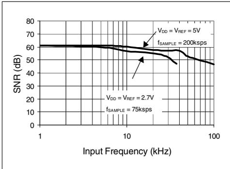
**FIGURE 2-20:** Signal to Noise (SNR) vs. Input Frequency.
