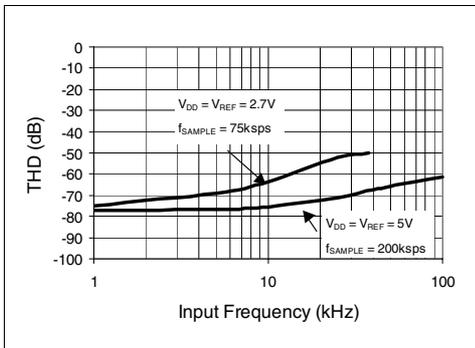
**FIGURE 2-21:** Total Harmonic Distortion (THD) vs. Input Frequency.
