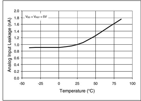
**FIGURE 2-39:** Analog Input Leakage Current vs. Temperature.
