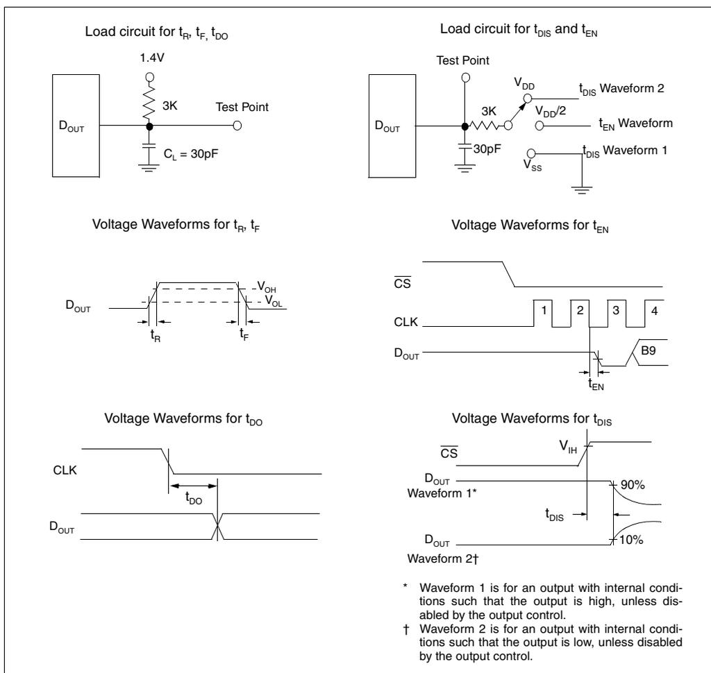
**FIGURE 1-2:** Test Circuits.
