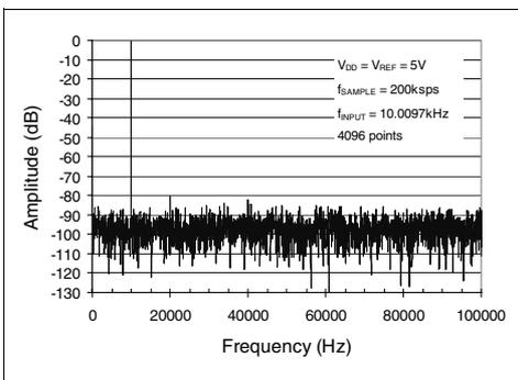
**FIGURE 2-27:** Frequency Spectrum of 10kHz input (Representative Part).
