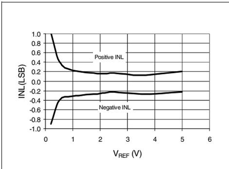
**FIGURE 2-2:** Integral Nonlinearity (INL) vs.  $V_{REF}$ .
