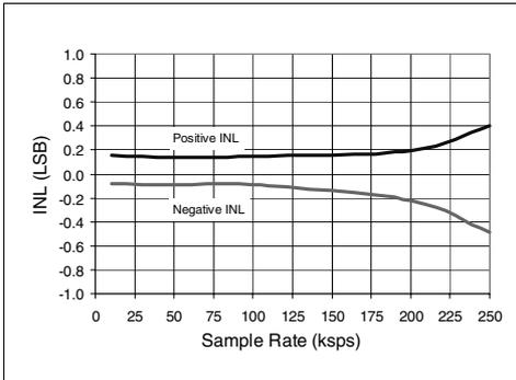
**FIGURE 2-1:** Integral Nonlinearity (INL) vs. Sample Rate.
