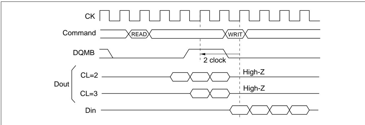
**Same bank, different ROW address:** When the ROW address changes, consecutive write commands cannot be executed; it is necessary to separate the two commands with a precharge command and a bank-active command.
