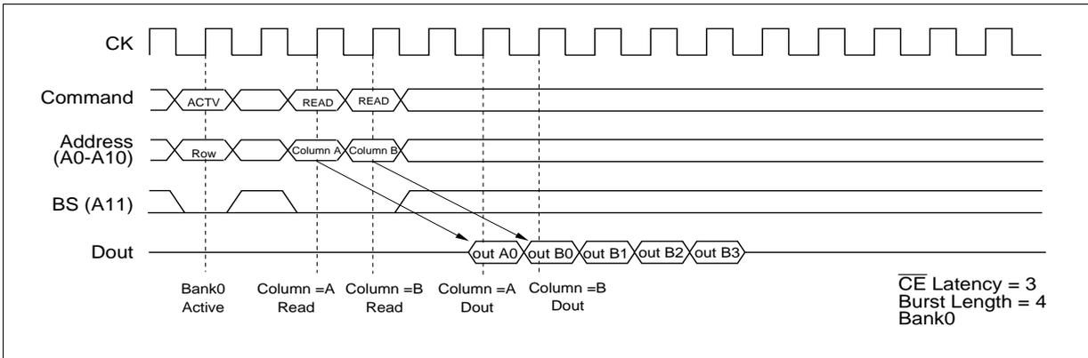
**Same bank, different ROW address:** When the ROW address changes on same bank, consecutive read commands cannot be executed; it is necessary to separate the two read commands with a precharge command and a bank-active command.
