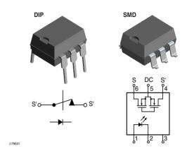
structed as a multi-chip hybrid device. Actuation control is via an Infrared LED. The output switch is a combination of a photodiode array with MOSFET switches and control circuity. The relays can be configured for AC/DC or DC only operation.
