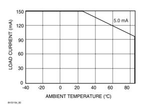
Fig. 1 Recommended Operating Conditions
