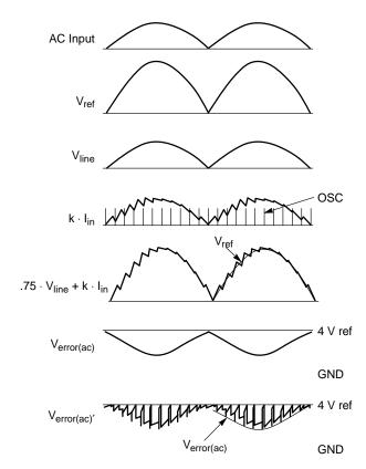
Figure 31. Typical Signals for PFC Circuit
