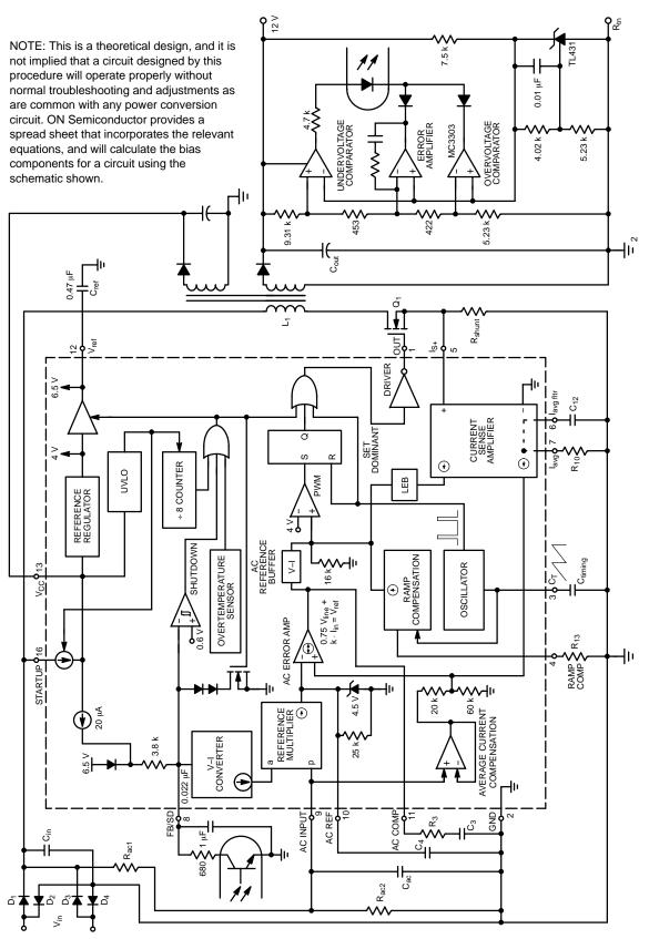
Figure 38. Typical Application Schematic
