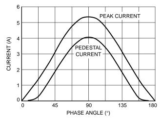
Figure 39. Switching Current versus Phase Angle
