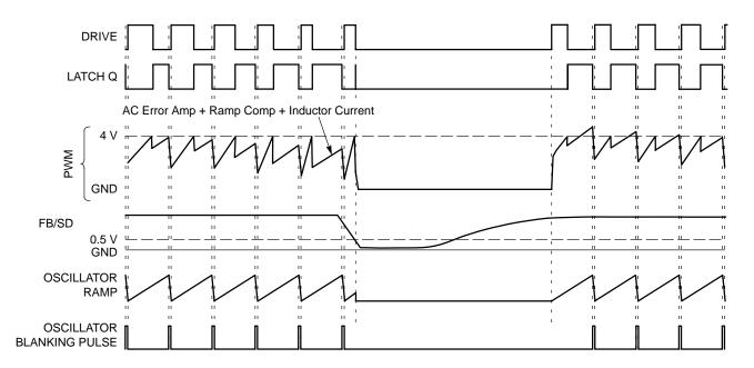
Figure 2. Switching Timing Diagram
