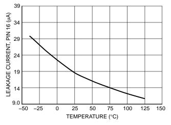
Figure 9. Startup Leakage versus Temperature
