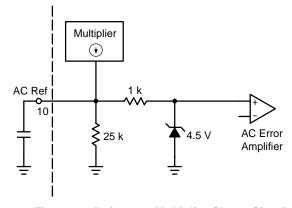
Figure 34. Reference Multiplier Clamp Circuit
