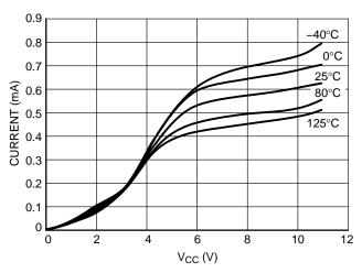
Figure 6. Bias Current in Shutdown Mode
