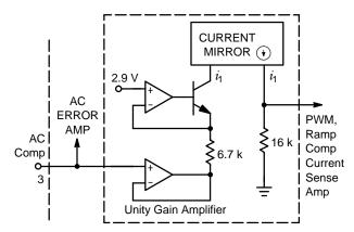
Figure 37. AC Reference Buffer Schematic
