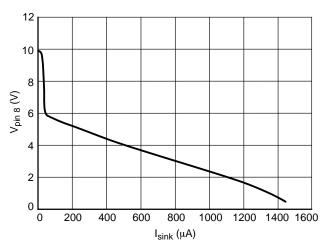
Figure 5. FB/SD V-I Characteristics
