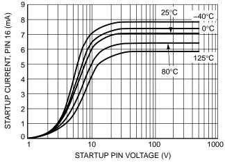
Figure 8. Startup Current versus High Voltage
