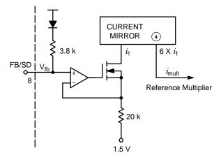
Figure 33. Multiplier V-I Converter
