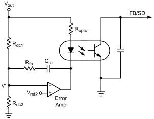
Figure 41. Error Amplifier Circuit
