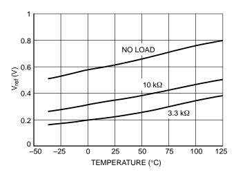
Figure 22. V<sub>ref</sub> in Shutdown Condition
