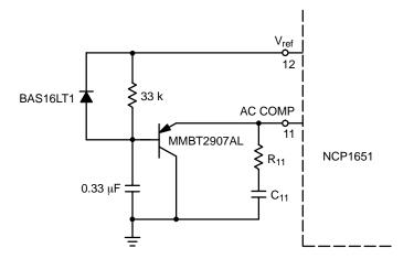
Figure 24. Soft Start Circuit
