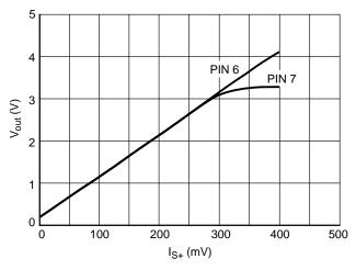
Figure 4. Current Sense Amplifier Gain
