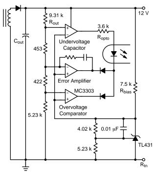
Figure 42. Error Amp with Over/Undershoot Protection
