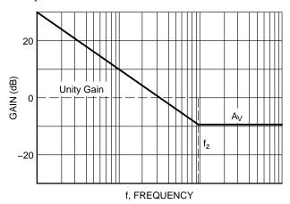
Figure 44. Pole-zero Bode Plot
