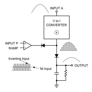
Figure 32. Simplified Multiplier Schematic
