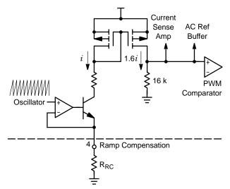
Figure 35. Ramp Compensation Circuit
