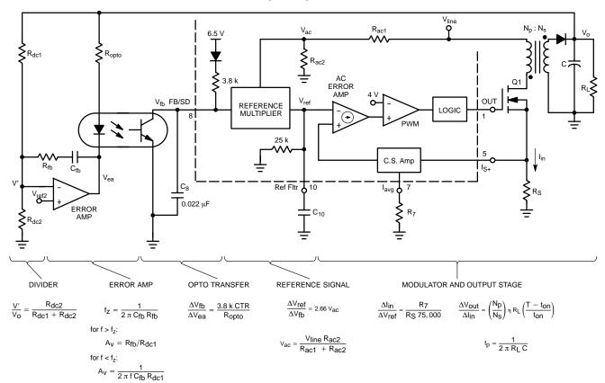
Figure 43. Voltage Regulation Loop
