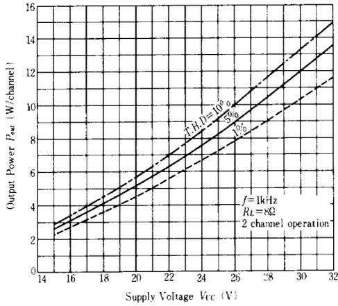
**OUTPUT POWER VS. SUPPLY VOLTAGE (2)**
