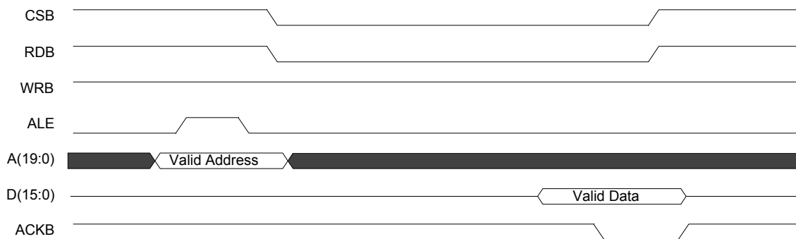
Figure 114 Microprocessor Read Access with ALE
