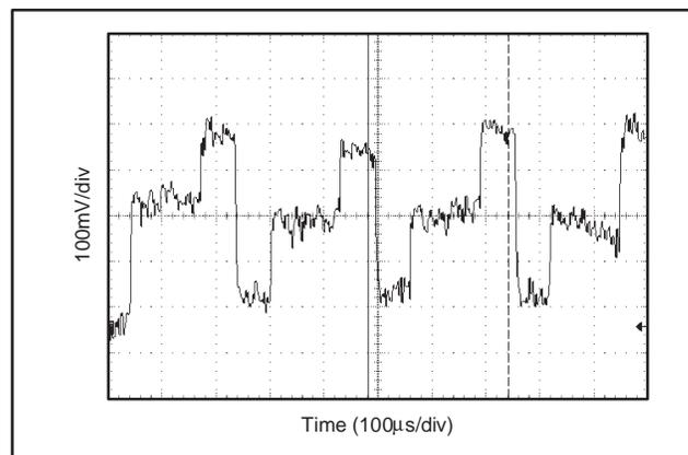
Figure 8.  $V_{OUT}$  Clock Feedthrough Glitch, Coarse Offset Adjust = 59mV, Gain = 1152, CLK\_CFG = '00' (default).  $V_{OUT}$  Glitch (RTI) = 347 $\mu$ V<sub>PP</sub>.
