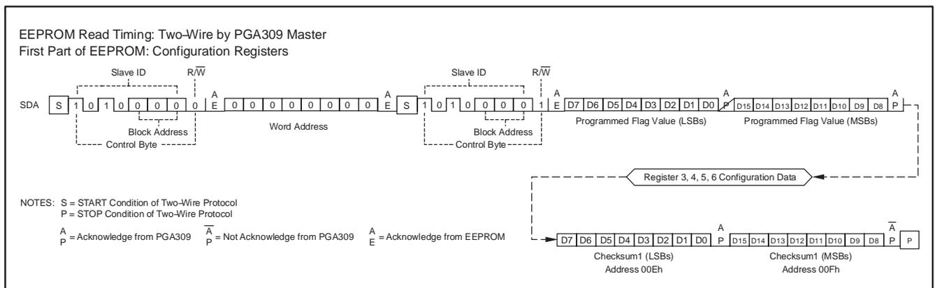
Figure 53. First Part of External EEPROM Timing for Stand-Alone Mode
