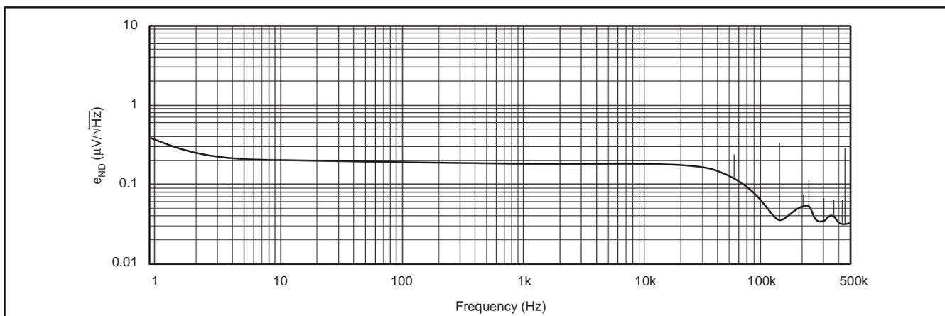
Figure 12.  $V_{OUT}$  Noise Spectrum for Coarse Offset Adjust =  $-56\text{mV}$ , Gain = 1152,  $V_{IN} = +57\text{mV}$ , CLK\_CFG = '01'.
