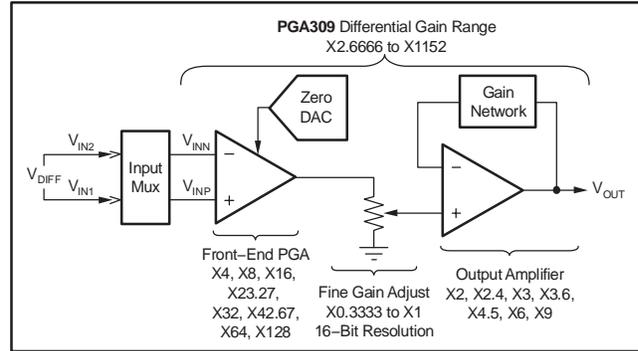
Figure 2. Gain Blocks of the PGA309
