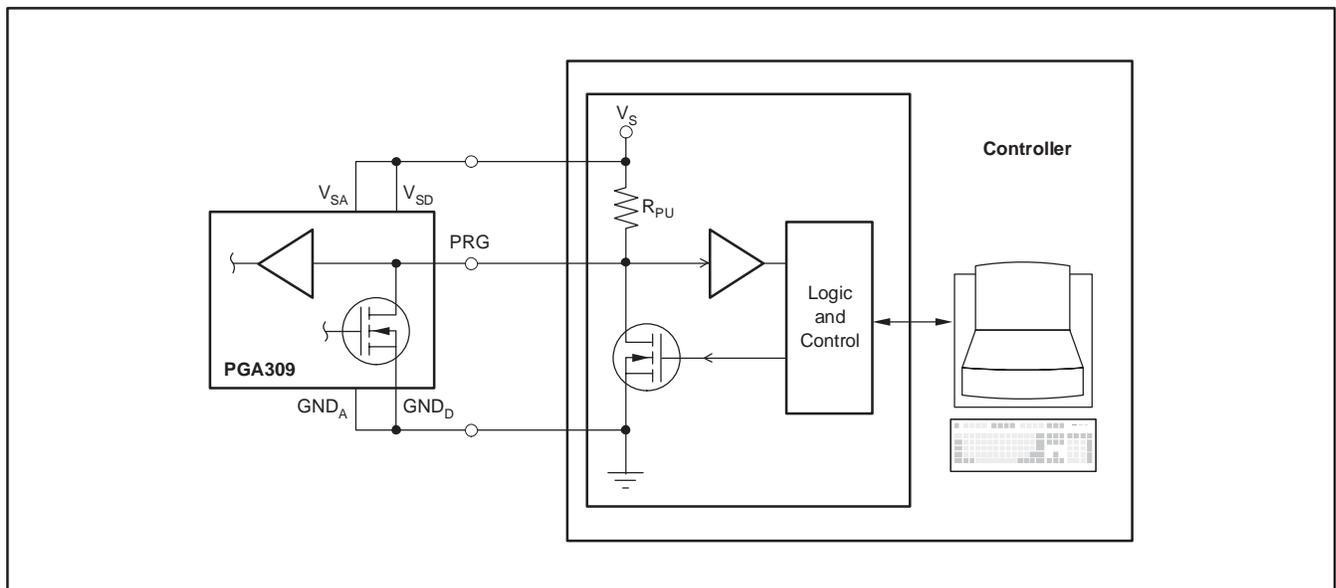
Figure 47. Typical PGA309 PRG To Controller Connection
