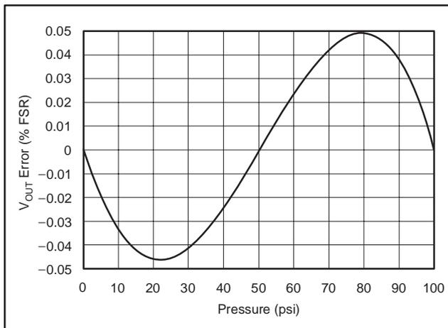
Figure 29. Parabolic Bridge Corrected Nonlinearity vs Pressure
