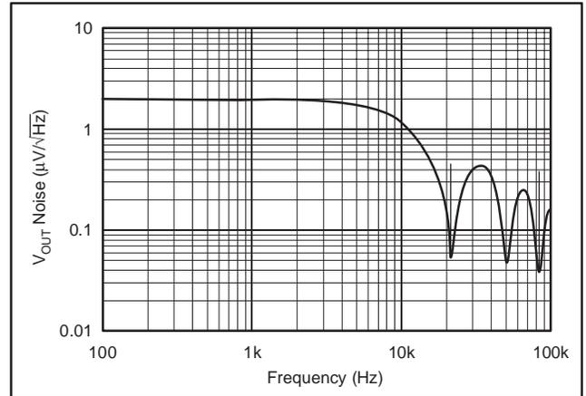
Figure 16.  $V_{OUT}$  Noise Spectrum for Coarse Offset Adjust =  $-56\text{mV}$ , Gain = 1152,  $V_{IN} = +57\text{mV}$ , CLK\_CFG = '11'.
