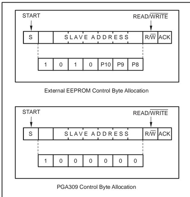
Figure 45. External EEPROM and Control Byte Allocation
