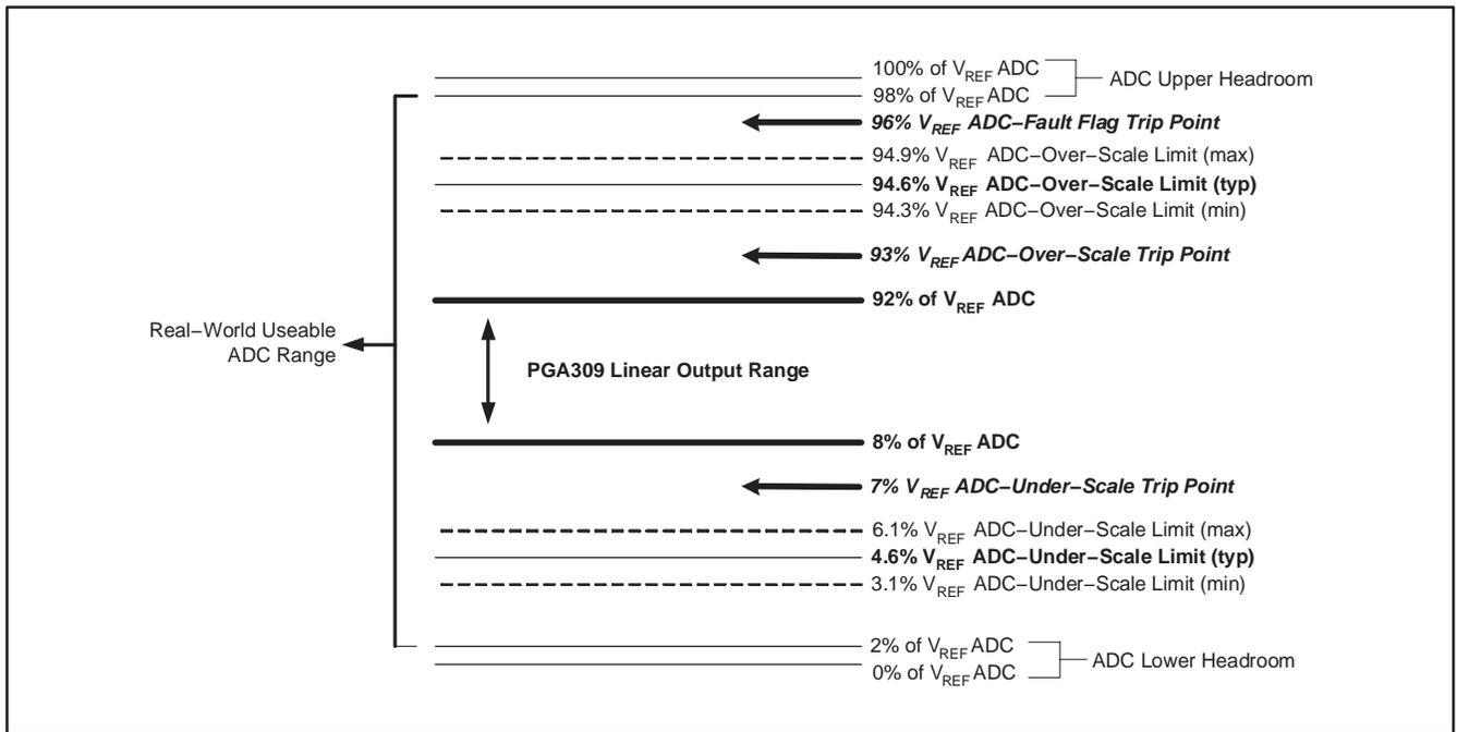
Figure 23. System ADC Range Budget for Over-Scale, Under-Scale, and Linear Output
