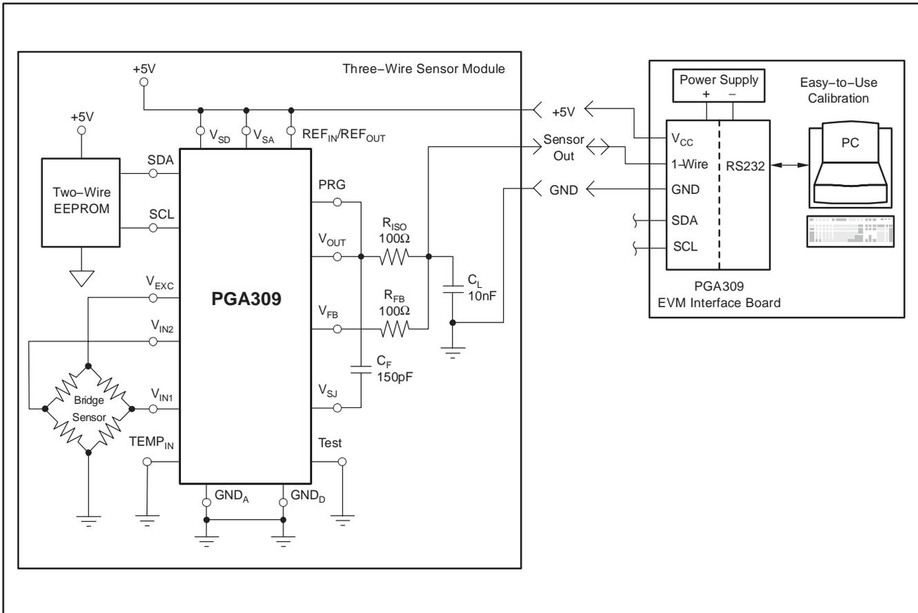
Figure 57. One-Wire Operation with PRG Tied to V<sub>OUT</sub>
