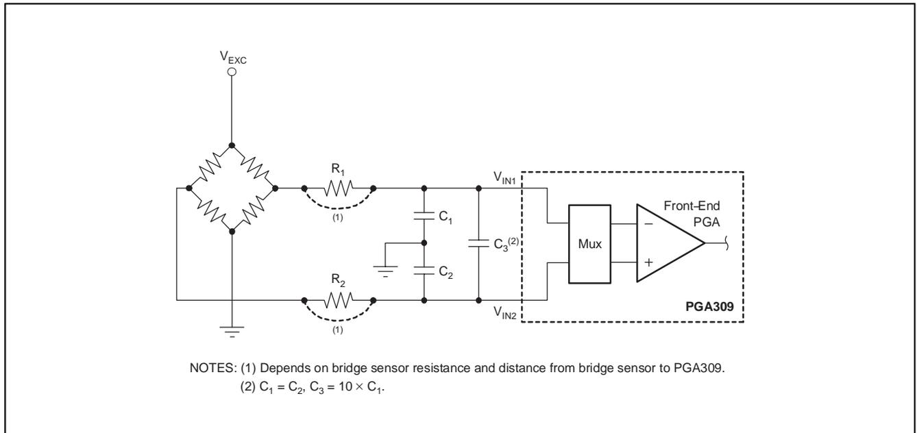
Figure 40. Input Filtering
