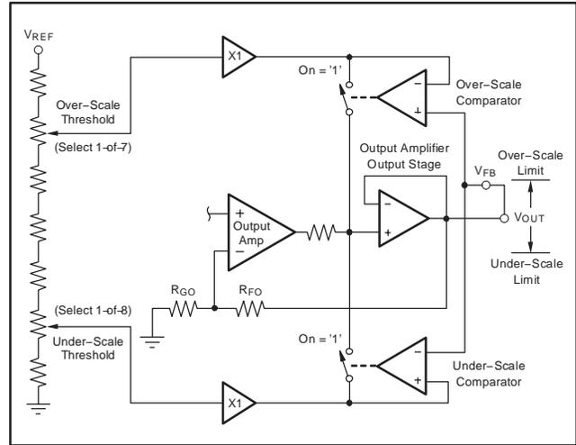
Figure 21. Over-Scale and Under-Scale Limit Circuit
