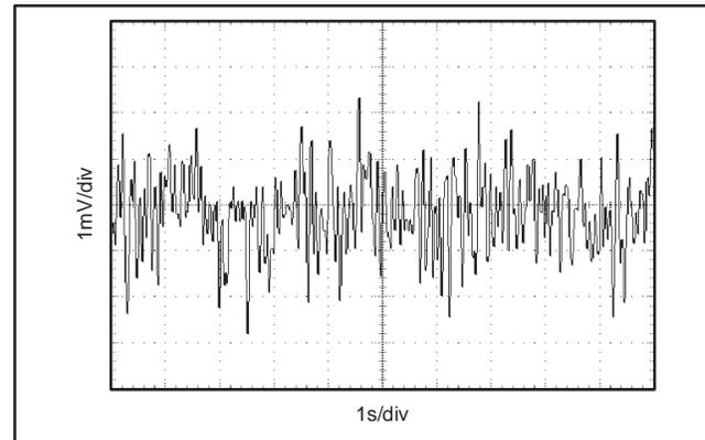
Figure 11. 0.1Hz to 10Hz  $V_{OUT}$  Peak-to-Peak Noise for Coarse Offset Adjust =  $-56\text{mV}$ , Gain = 1152,  $V_{IN} = +57\text{mV}$ , CLK\_CFG = '01',  $V_{NPP}$  (RTI) =  $4.44\mu\text{Vpp}$ .
