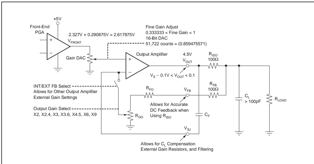
Figure 4. Fine Gain Adjust of the PGA309
