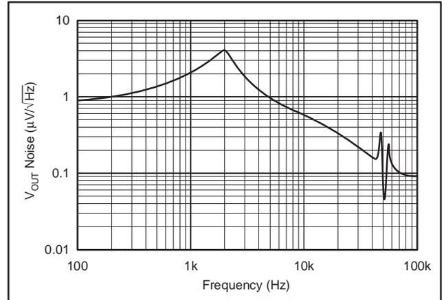
Figure 15.  $V_{OUT}$  Noise Spectrum for Coarse Offset Adjust =  $-56\text{mV}$ , Gain = 1152,  $V_{IN} = +57\text{mV}$ , CLK\_CFG = '10'.
