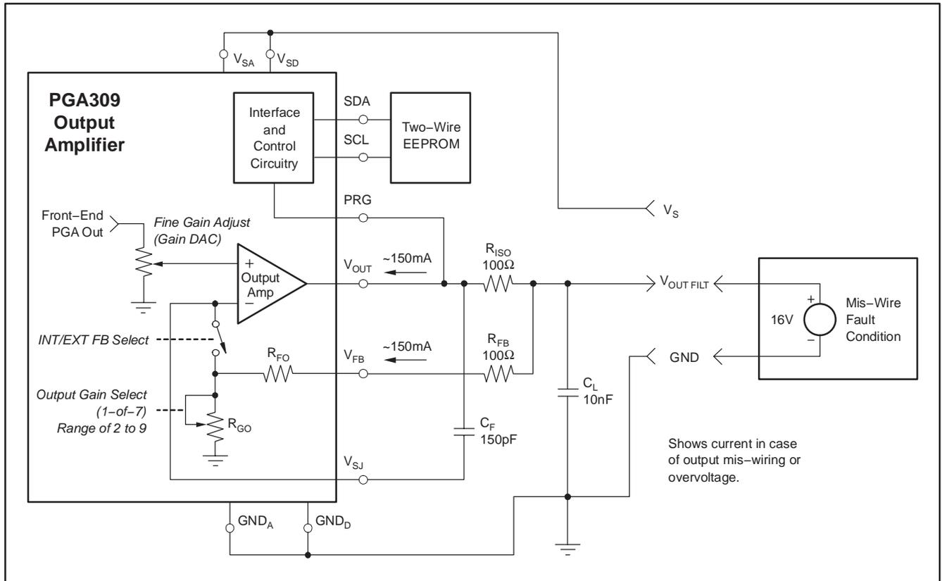
Figure 37. Output Amplifier in a Common 3–Terminal Sensor Application
