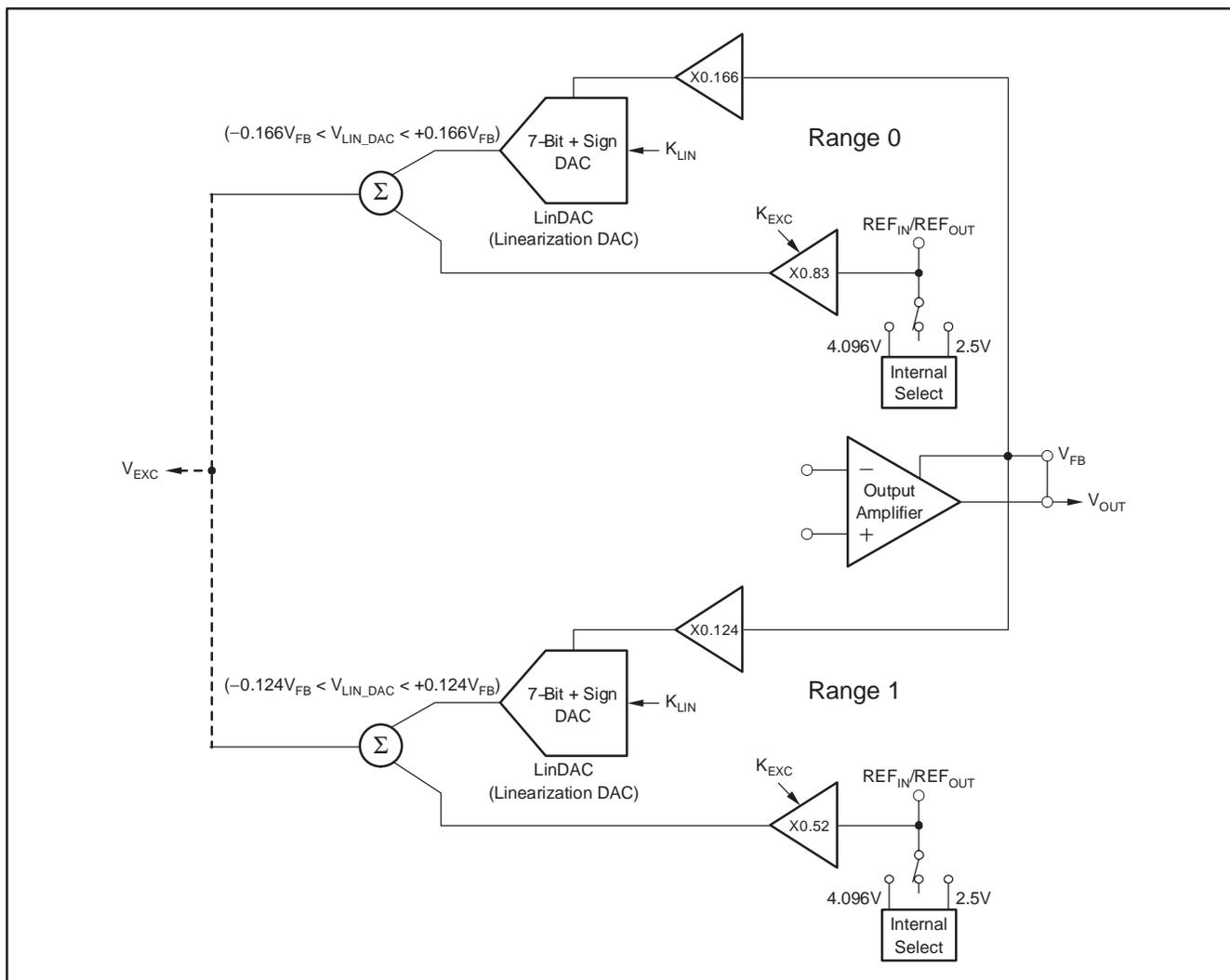
Figure 26. Linearization Circuitry
