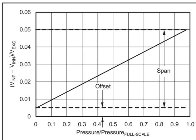
Figure 60. Example of Span and Offset
