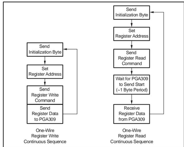
Figure 49. One-Wire Access to PGA309 Registers
