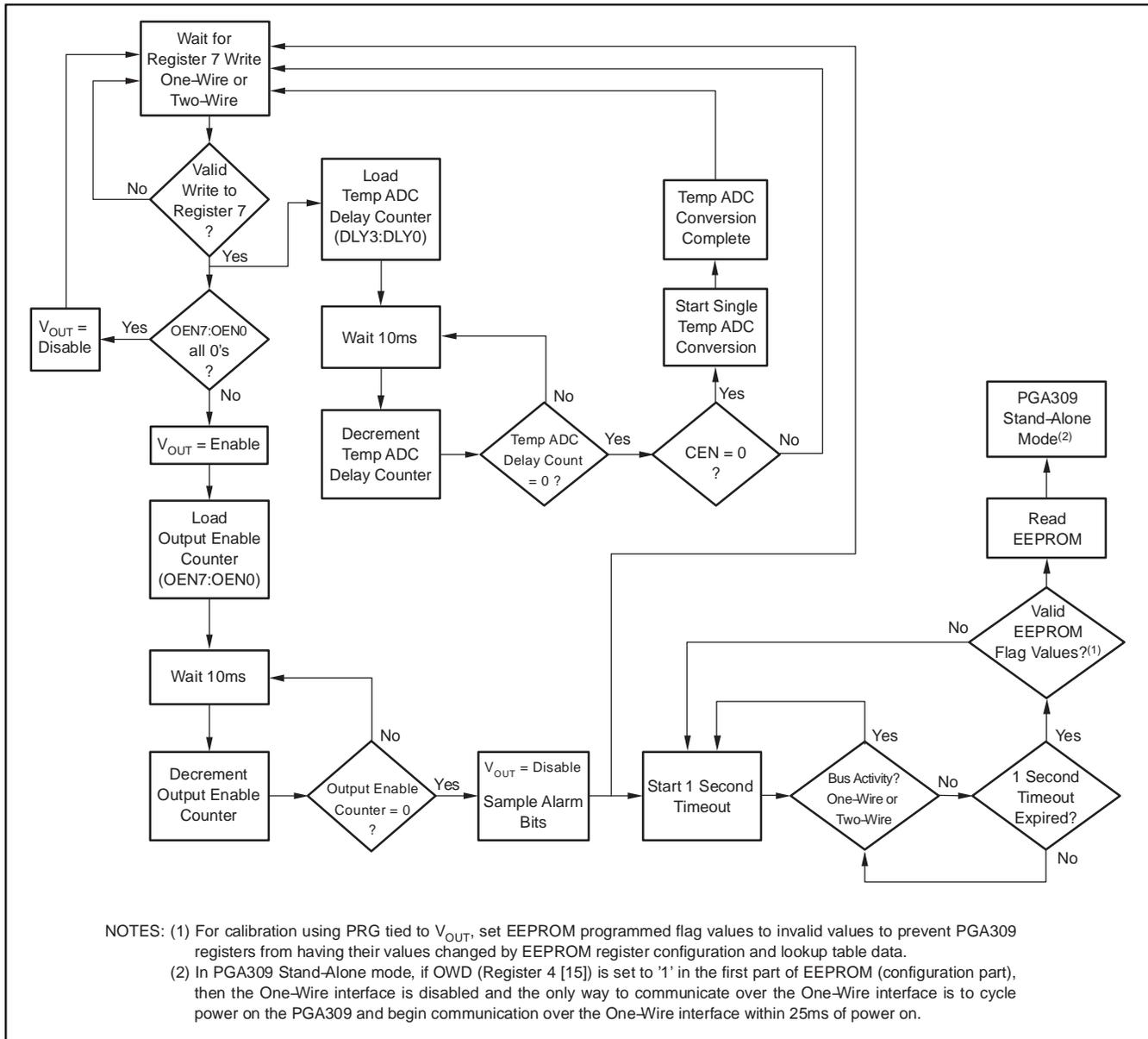
Figure 58. Output Enable/Disable State Machine
