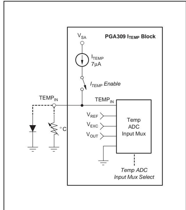
Figure 32. I<sub>TEMP</sub> for External Temperature Measurement
