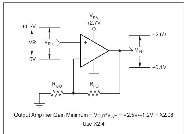
Figure 39. Output Amplifier Minimum Gain at Low Supply
