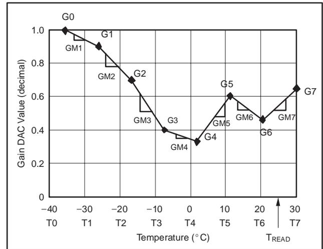
Figure 18. Gain DAC Temperature Coefficients—Definition Example
