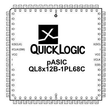
Pins identified I/SCLK, SM, SO and SI are used during scan path testing operation.
