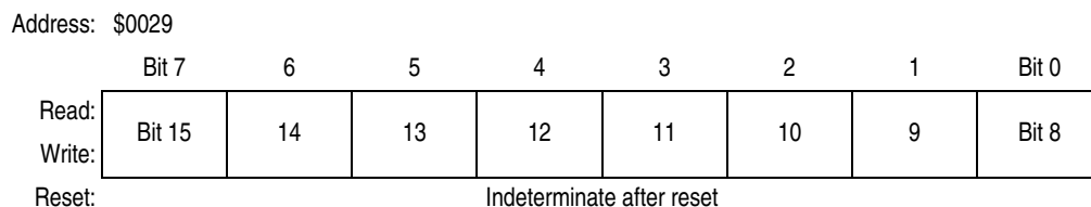
Figure 18-15. TIM Channel 1 Register High (TCH1H)
