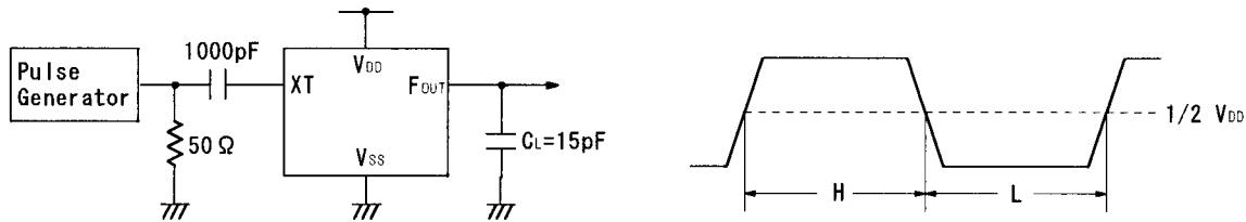
(2) Output Signal Rise/Fall Time ( $C_L=15pF$ )
