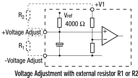
$$V1_A = \frac{V1 \times R1}{R1 + 4000} \text{ where } V_{ext} = \frac{4000 \times V1_A}{V1 - V1_A}$$
