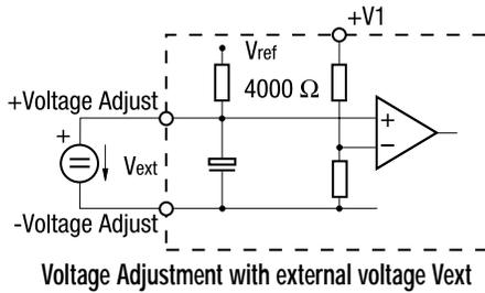
$$V1_A = \frac{V_{ext} \times V1}{2.5V} \text{ where } V_{ext} = \frac{2.5V \times V1_A}{V1}$$
