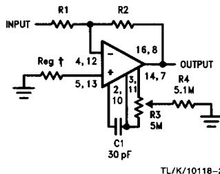
†May be zero or equal to parallel combination of R1 and R2 for minimum offset.
