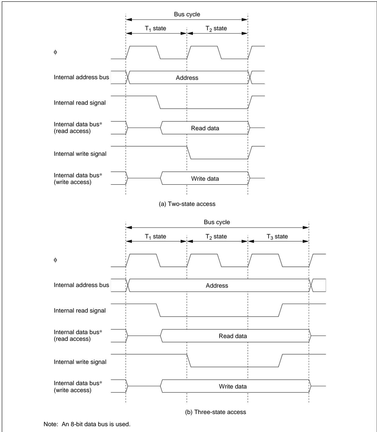
**Figure 4-2. On-Chip Peripheral Module Access Cycle**
